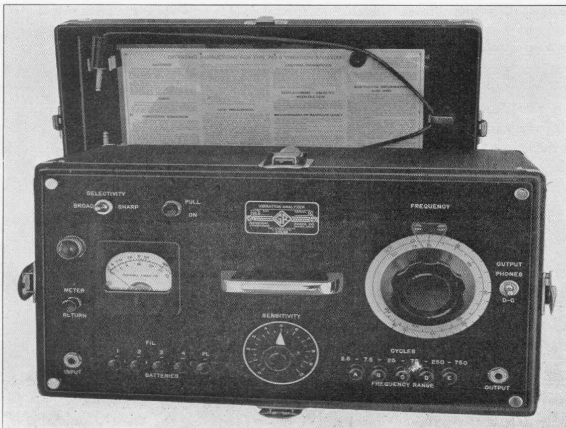
FIGURE 1. Panel view of the TYPE 762-B Vibration Analyzer.
