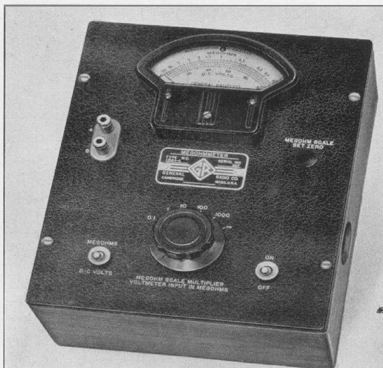
FIGURE 1. Panel view of the TYPE 1861-A Megohmmeter. Superseding the TYPE 487-A, this new instrument measures resistances from 2000 ohms to 50,000 megohms and can also be used as a d-c voltmeter.
